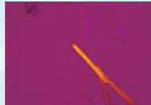
Amosite Positive: Subtractive diagonal position
