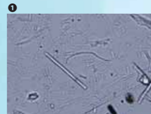
Chrysotile and amosite (refraction index of the liquid nD = 1.605, CFI P Achromat 40x)
