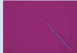
Crocidolite Negative: Additive diagonal position
